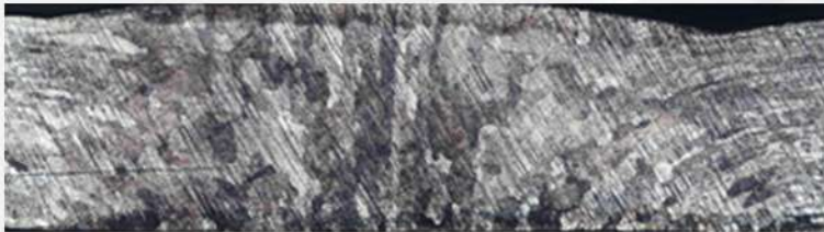
Fig. 4 - Structure of TIG welded GSP part without any porosity
