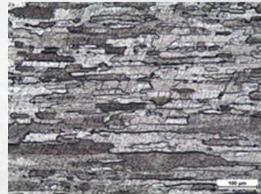
Fig. 2 – GSP with fine interlocked grains of high aspect ratio, which possess good resistance against
